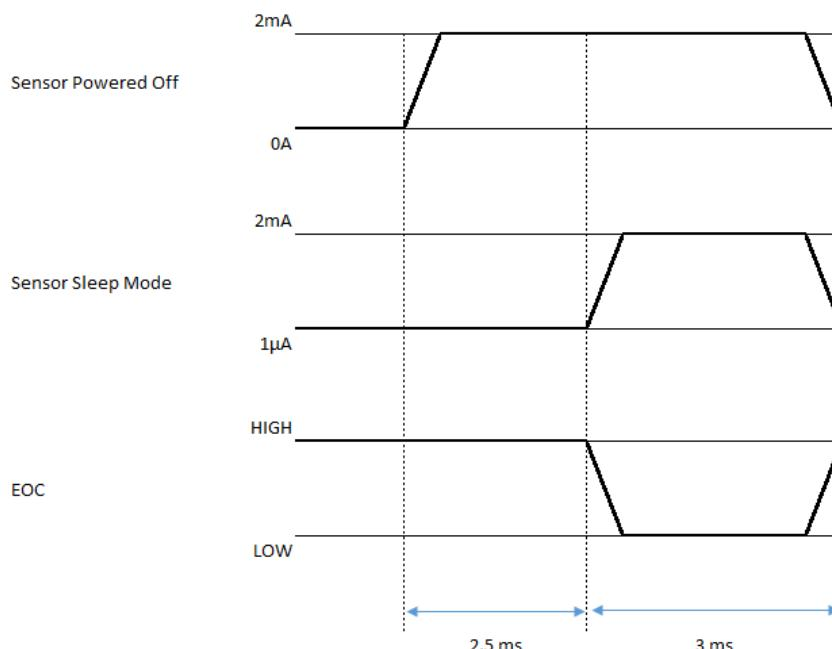
Time until the pressure and temperature value is available after the request by the I<sup>2</sup>C master:
