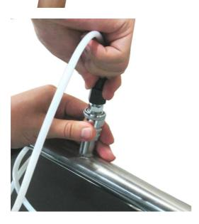
3. Connect the quick coupling at the other end of the teflon hose to the process.
