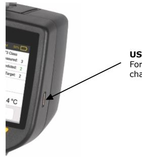
**USB-C connector** For data transfer and device charging
