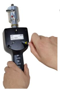
1. Open the two screws at the back of the instrument.
