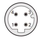
4-pole connector, male (View onto the connector)
