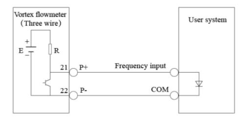
Parallel connection method digital output connection
