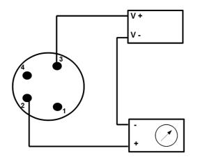
2 Wires (loop powered)
