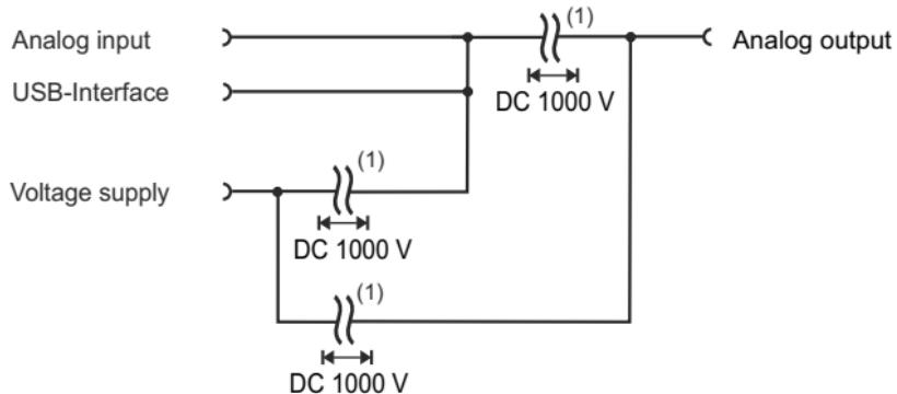
(1) The voltage of von DC 1000 V between the circuit parts is a test voltage and has not to be seen as a continuous voltage to be applied.
