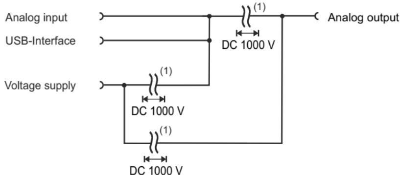
(1) The voltage of von DC 1000 V between the circuit parts is a test voltage and has not to be seen as a continuous voltage to be applied.
