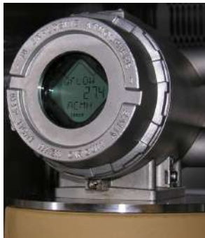
Figure 1-3: Transmitter electronics enclosure with optional local display and glass endcap
