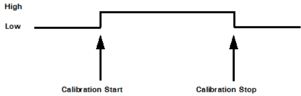
Figure 4-12: Gating configuration parameter State gated, active high
