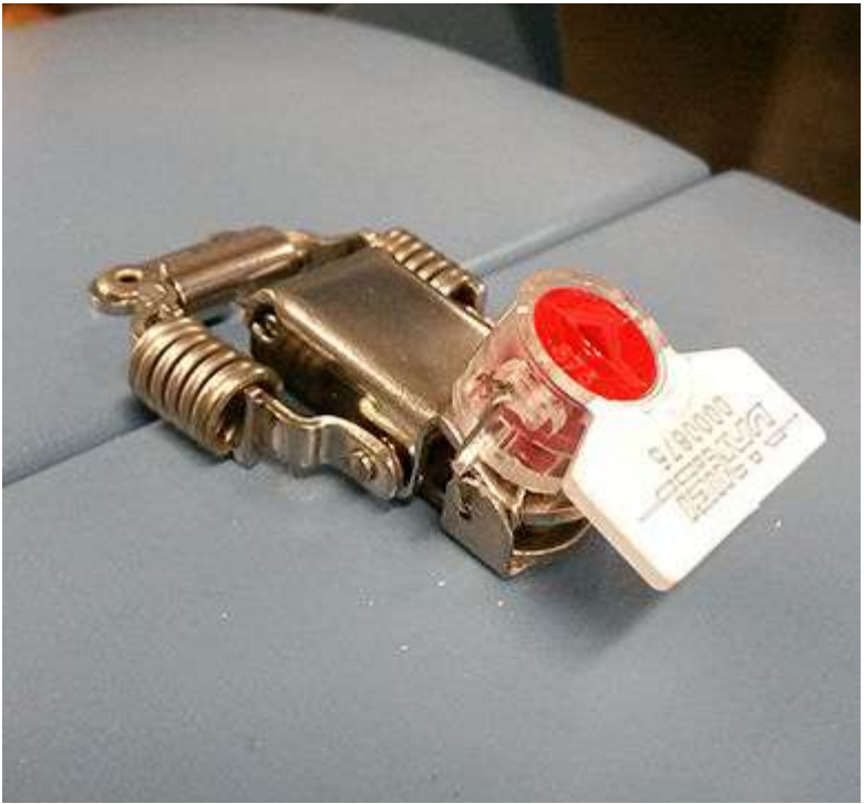
Figure 3-12: Shroud latch with Security seal
