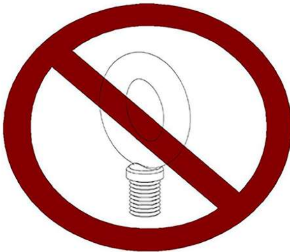
Figure 2-12: Non-compliant eye bolt
