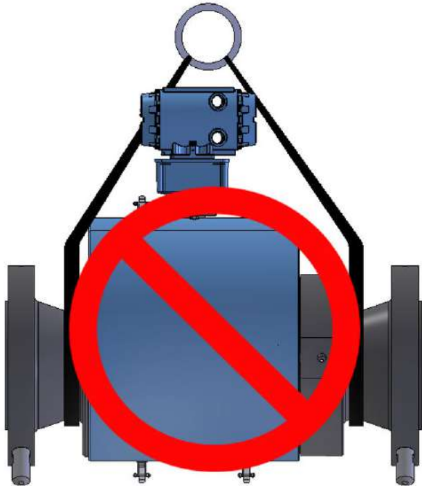
Figure 2-16: Incorrect sling attachment
