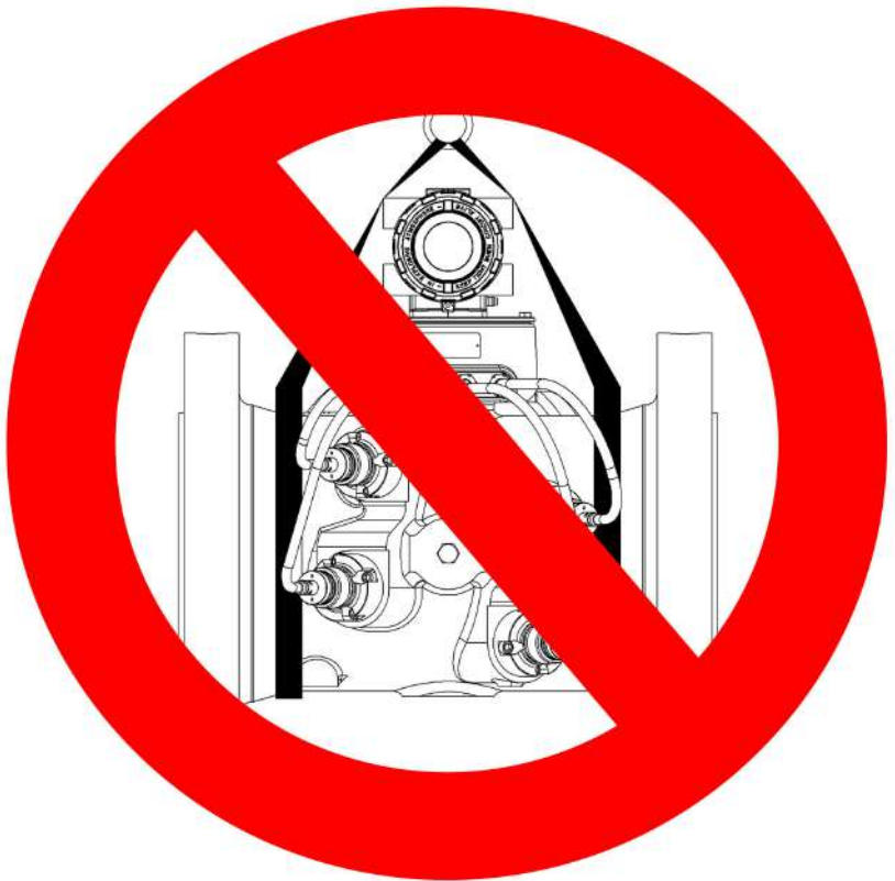
Figure 2-16: Incorrect sling attachment
