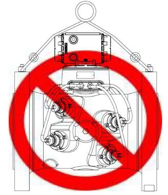
Figure 2-14: Incorrect sling attachment
