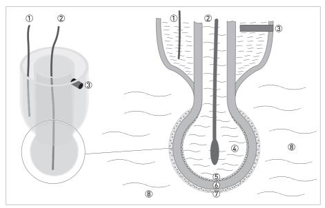
Figure 1-1: Measuring principle for pH measurement
