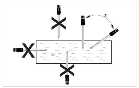
Figure 3-2: Installation requirements
