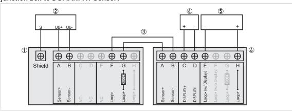
Figure 4-4: Example of connecting the SMARTMAC 200 W to a control system without internal 250  $\Omega$  resistor and one additional loop powered device.
