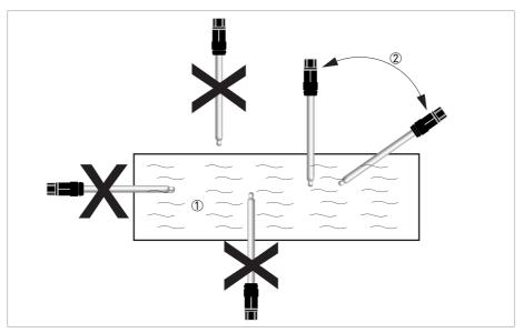
Figure 3-2: Installation requirements
