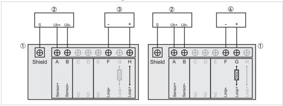
Figure 4-5: SMARTMAC 200 W connection to a control system with internal 250  $\Omega$  resistor (left side). SMARTMAC 200 W connection to a control system without internal 250  $\Omega$  resistor (right side).
