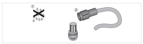
Figure 4-1: Connecting the cable to the sensor
