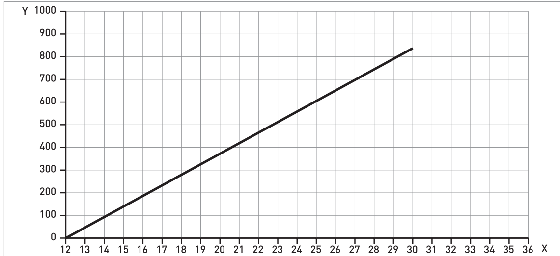
Figure 2-5: Minimum power supply voltage for an output of 21.5 mA at the terminals (Non-Ex and Hazardous Location approval (Ex i / IS))
