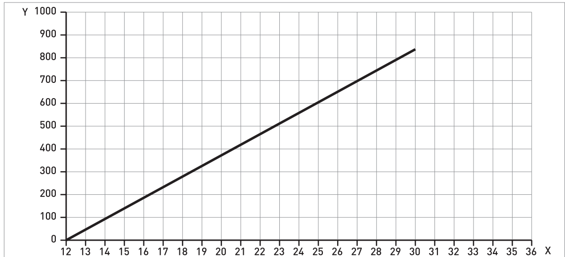
Figure 2-3: Minimum power supply voltage for an output of 21.5 mA at the terminals
