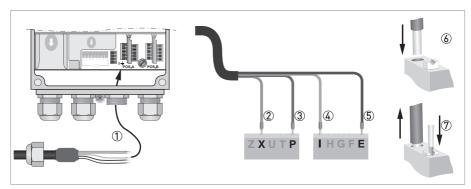
Figure 4-4: Connecting the sensor cable to the signal converter
