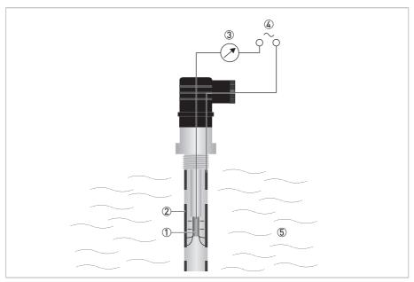
Figure 1-1: Measuring principle for conductivity measurement
