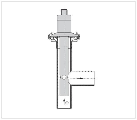
Figure 3-1: Mounting position
