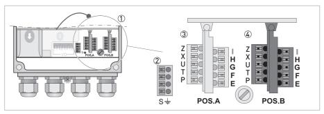
Figure 4-3: Junction of the signal converter
