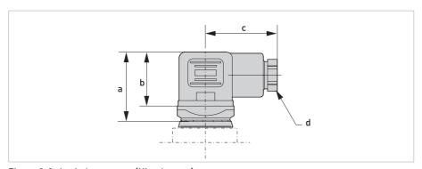
Figure 2-2: Angled connector (Hirschmann)
