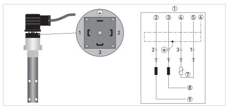
Figure 4-2: Cable assign of a Hirschmann plug
