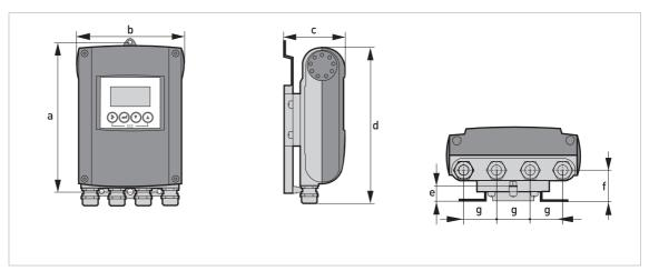
Figure 2-1: Dimensions die-cast aluminium housing
