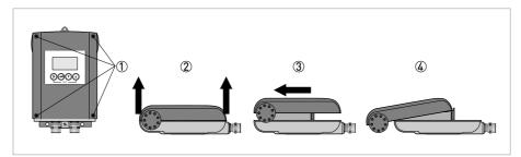
Figure 4-1: Opening the converter housing
