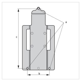
Figure 2-3: Dimensions mounting plate
