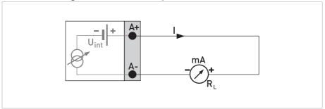
Figure 4-6: Current output (active)
