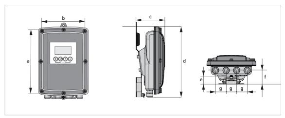
Figure 2-2: Dimensions stainless steel housing
