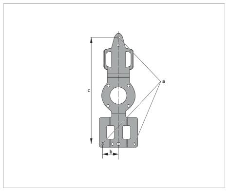
Figure 2-4: Dimensions mounting plate
