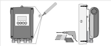
Figure 3-1: Mounting procedure to walls
