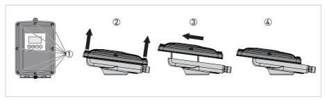
Figure 4-2: Opening the converter housing
