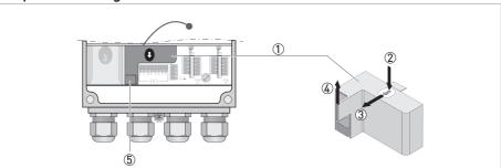
Figure 4-10: Removing the cover
