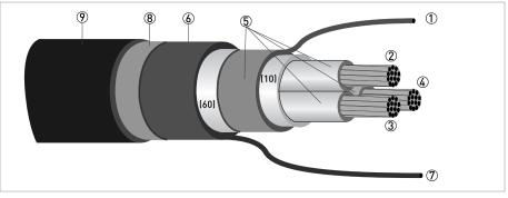
Figure 4-2: Construction of signal cable A (armoured version)
