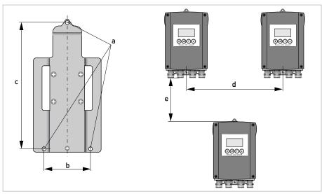
Figure 3-2: Wall mounting of multiple devices (aluminium housing)
