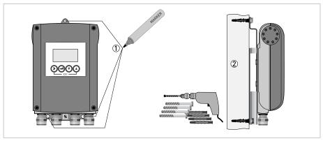
Figure 3-1: Mounting the wall-mounted housing
