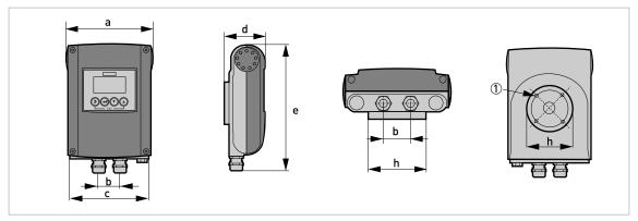
Figure 2-3: Dimensions of compact 0° version, aluminium housing 4 x M 6
