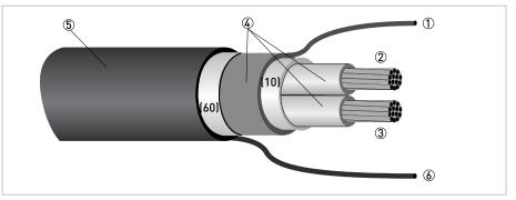
Figure 4-1: Construction of signal cable A (standard version)
