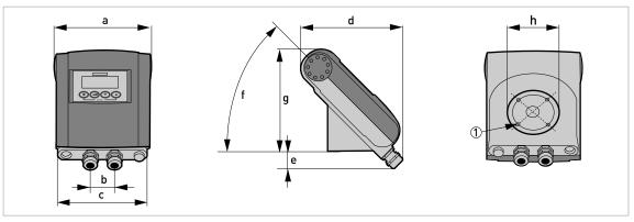
Figure 2-4: Dimensions of compact 45° version, aluminium housing 4 x M 6
