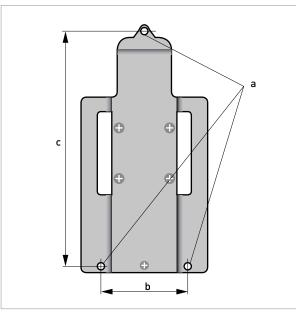
Figure 2-5: Dimensions of mounting plate of wall-mounted version, aluminium housing
