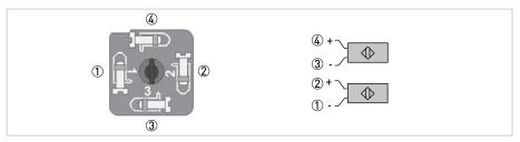
Figure 4-2: Electrical connection of NAMUR limit switches K1/K2
