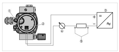
Figure 4-7: Electrical connection of ESK3x
