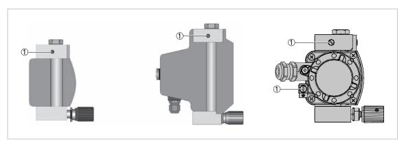
Figure 4-10: Grounding connections
