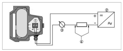
Figure 4-8: Electrical connection M8E
