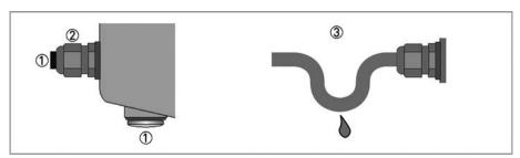
Figure 4-11: Cable feedthrough
