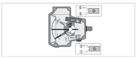
Figure 4-4: Electrical connection of NAMUR limit switches K1/K2
