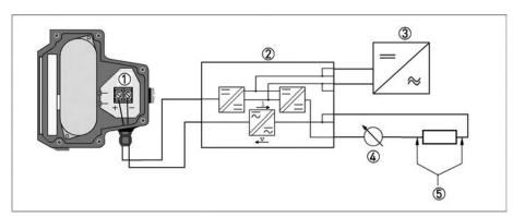
Figure 4-9: Electrical connection with galvanic isolation
