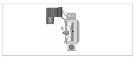
Figure 4-6: Settings of REED limit switch
