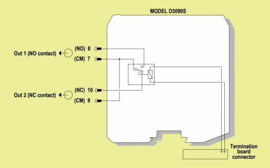
Relay contacts shown in de-energized position. Terminals 7-8 are open; terminals 9-10 are closed.
