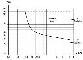
DC and AC Load breaking capacity:
