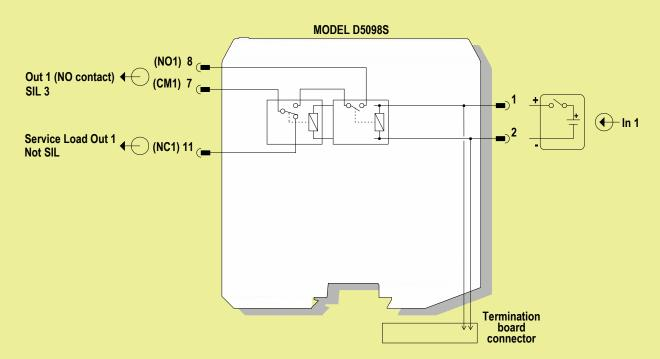
Relay contacts shown in de-energized position. Terminals 7-8 are open; terminals 7-11 are closed.
