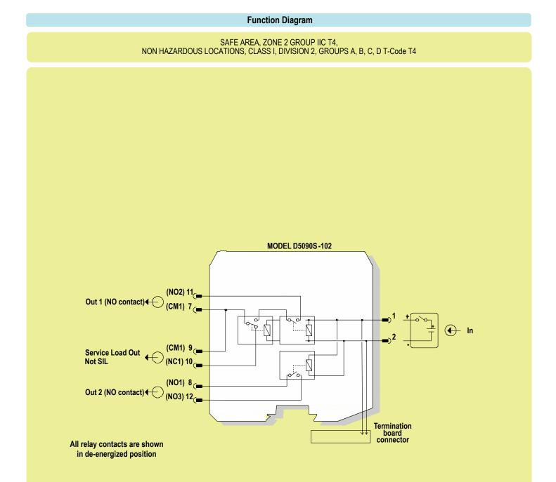
To prevent relay contacts from damaging, connect an external protection (fuse or similar), chosen according to the relay breaking capacity diagram.
