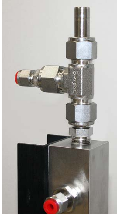
Figure 3-2 Port Connector for Polydisperse Aerosol Outlet
