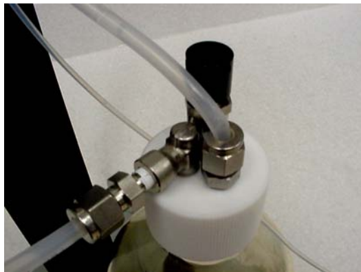
Figure 3-4 Bottle Cap Adapted for Nonrecirculation Mode
