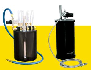
TSI's Oil Droplet Generators are a general-purpose atomizers that utilizes a Laskin nozzle to generate droplets for flow seeding. Pressurized air atomizes oil in the generator reservoir to produce the droplets. An internal impactor plate blocks large droplets from getting into the droplet stream exiting the device, allowing it to generate particles with a reasonably narrow size distribution.
