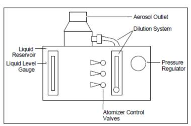
Figure 1: The Four Subassemblies of the Atomizer
