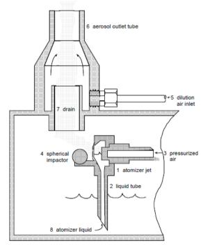
Figure 2: Schematic of the Atomizer
