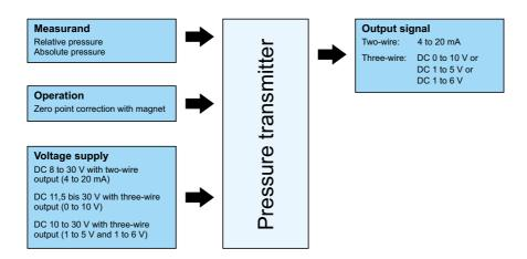
The approval stipulates use of the transmitter indoors only. All surfaces are made from stainless steel in the versions with electrical **connection 36** (round plug M12 × 1) and electrical **connection 75** (terminal head). These versions of the transmitter are also suitable for outdoor use.
